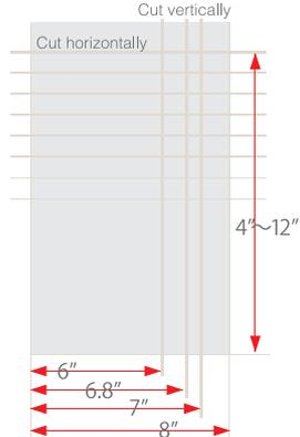
Move the built-in longitudinal cutter to four positions.
