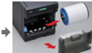
2. Remove the front panel door and insert the paper.
